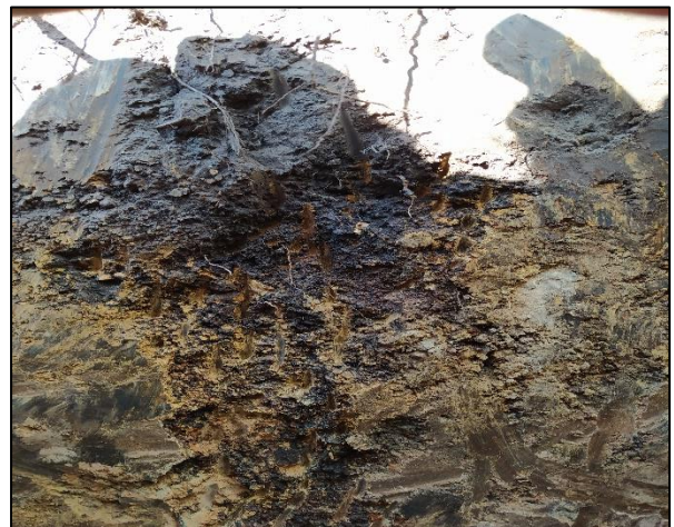
Plate 2: Ferricrete horizon extending into residual horizon
